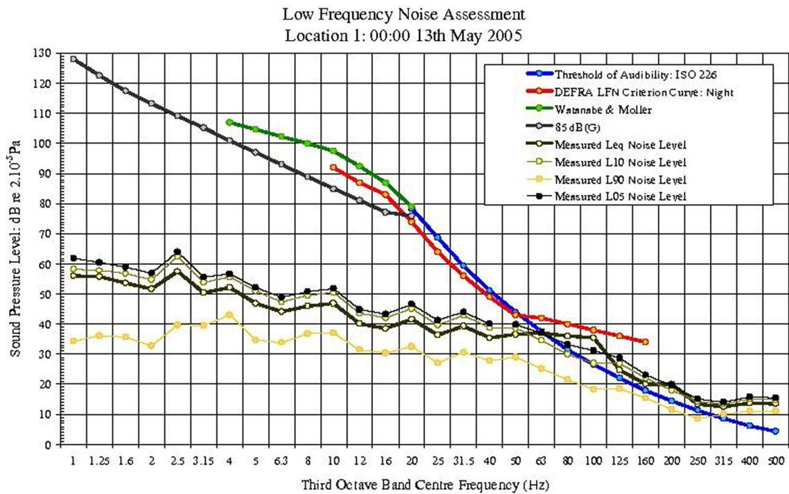
**Fig. 6** Typical wind farm-generated infrasound noise measurement inside of a dwelling [20]
