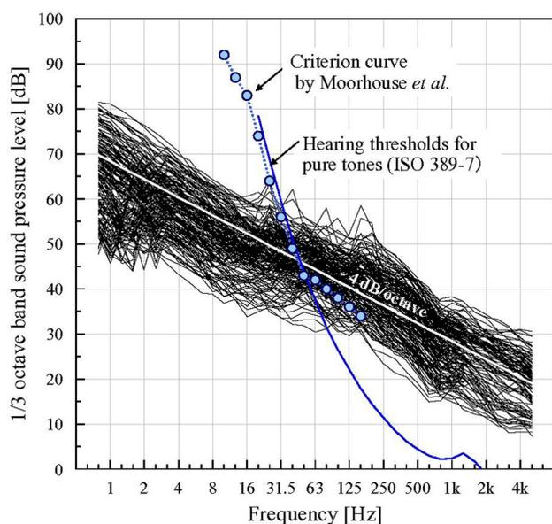
**Fig. 10** Measurement result of wind turbine noise levels at 164 points around 29 wind farms in Japan [42]
