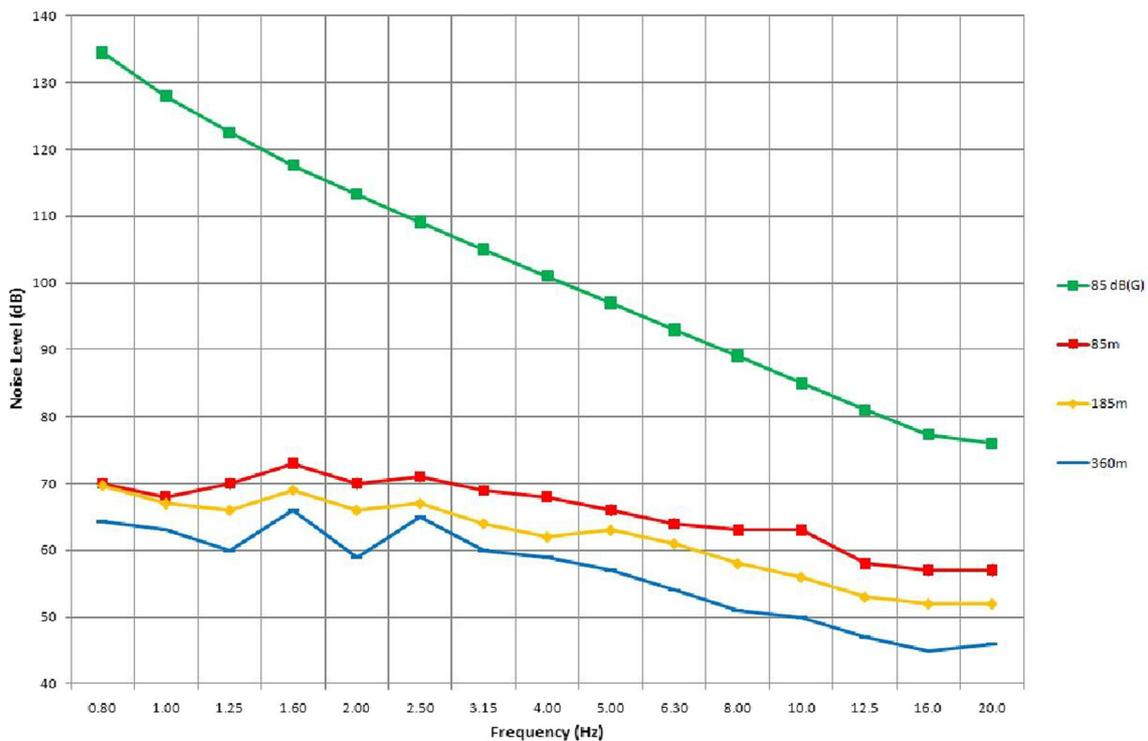
**Fig. 7** Measured levels of infrasound at Clements Gap Wind farm with a hub height wind speed of 6–8 m/s [39]
