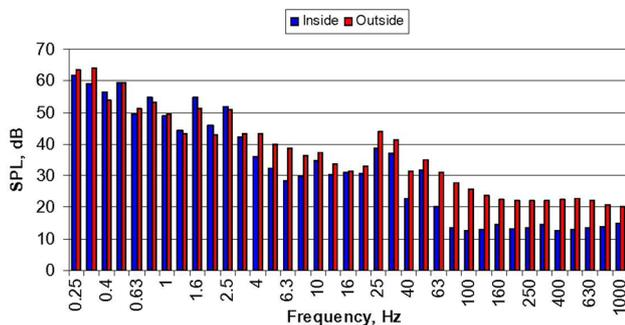
**Fig. 9** Waterloo Wind Farm one-third octave unweighted spectrum, downwind/crosswind wind speed 9.7 m/s, 16 rpm (blade pass frequency 0.8 Hz) [41]
