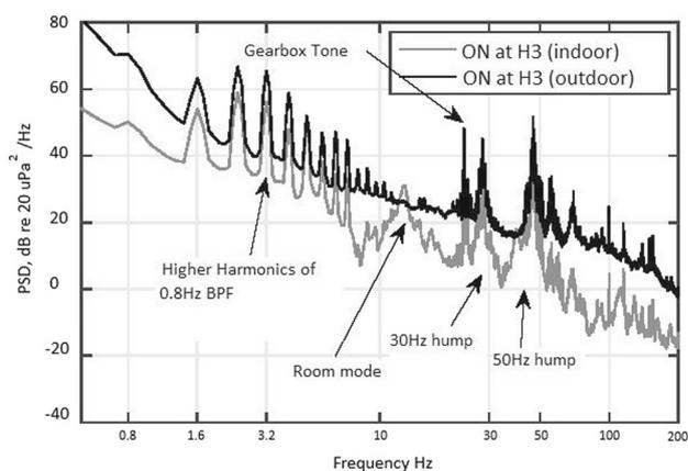
**Fig. 11** Comparison between the indoor/outdoor power spectral density (dwelling H3) [33]
