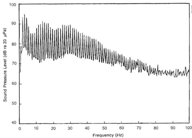
**Fig. 5** Average sound pressure level spectrum of MOD-1 measured at 107 m from the wind turbine (Figs. 3, 4; reference [13])
